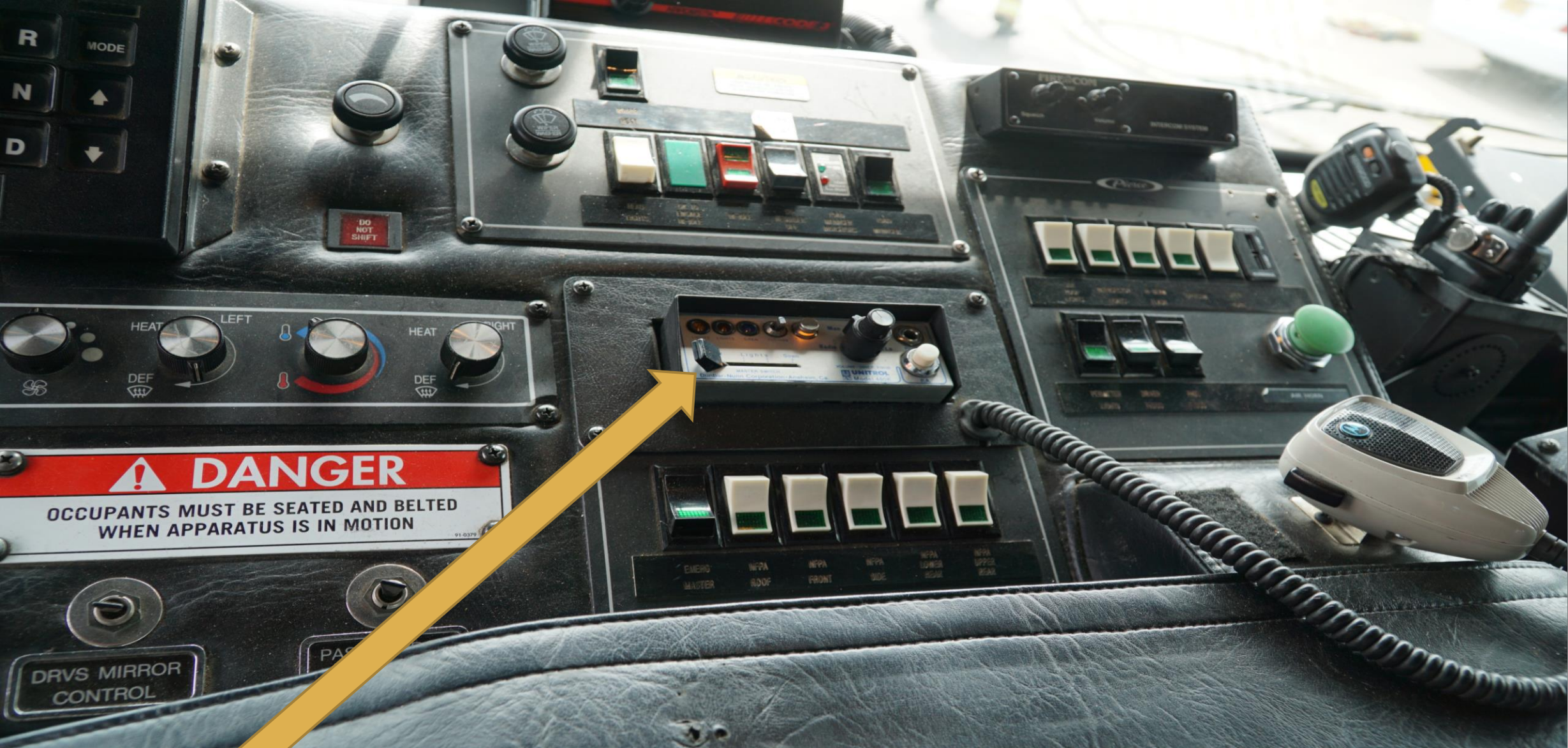
Emergency Master – Must be on for lights & slide lever over for lights
